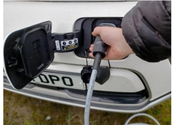
3. Charging the car – connecting to 4 Kw charging point
