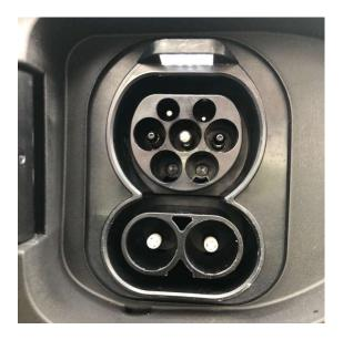
This is a CCS socket which will be on the Renault Kangoo. Think of this as your fuel port. There will be a way to open the charge port on any vehicle much the way you would do a petrol/diesel vehicle. Please remember to shut it after the cable has been removed.
