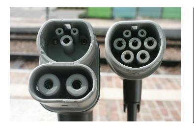
These are the two types of cable that will connect into the socket. A type 2 to type 2 cable (on the right of this image) should be supplied with each vehicle. This cable will connect from the charger to the socket on the fast-charging posts. The cable on the left is what is included on the tethered rapid charging units and plugs directly into the socket from the ChargePoint. It will be a thicker capable than the type 2 one.
